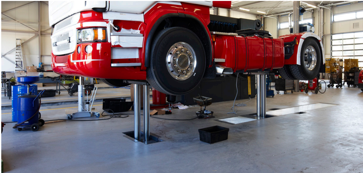
SCANIA - Peruwelz (TRUCKLIFT 2 cylindres).
